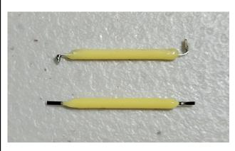
The lower LED is as received. The positive side of the LED has a tiny hole in the connector lead. The overall length of the LED is 1.15 inches.
