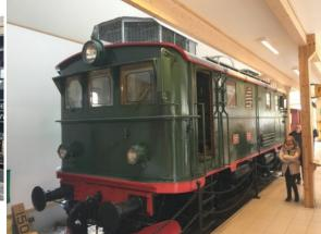
First loco used on newly electrified Flam Railway, vintage 1944. Because of the steep decent of the Flam line, this EL9 was delivered with a special braking system, the first locomotive delivered with electrical resistance brakes. In all, this loco had five different braking systems. Served on the Flam line until 1984.
