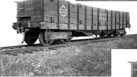
Original freight cars were simply flat cars, and started with just two axles anchored to the frame. The 2-axle pivoting truck developed by Jervis lead to similar under cars. Adding sides to the flatcar created the gondola.
