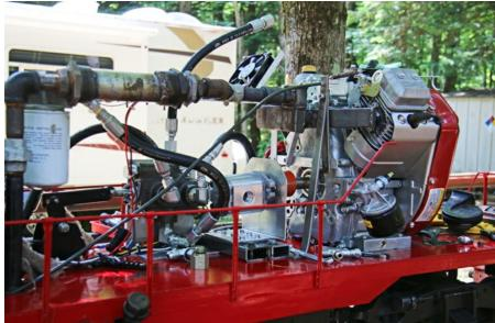
Engine insides: Inside is a v-twin, overhead-valve, gasoline engine coupled to a hydraulic pump, as these units have a hydraulic drive permitting speed regulation. The white filter is for the hydraulic fluid that is stored in the tank inside at the rear.
