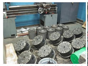
As part of the walk-through tour of the Amtrack Service Facility, visitors passed this lathe with some pictons and cylinder heads on the floor. Note the size compared to that green 5-gallon pail.
