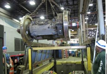
Above, the process begins by lifting the assembly and placing it on a lift that will lower it into the work area below the floor. There the carrige holding the assembly was moved sideways to a lift under the engine truck.
