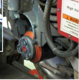
The axle is slowly raise into position in the support housing of the truck frame. A cover is then slid over the bearing. bolted to the frame shock and the attached to the cover.
