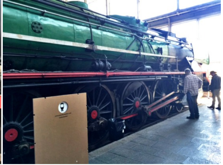
Road number 242F2009, newest steam loco in the museum, 4-8-4 Mikado built in 1956. In service until 1974. Mikados were unusual in Europe.
