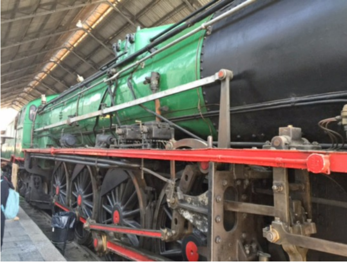
Road number 242F2009, newest steam loco in the museum, 4-8-4 Mikado built in 1956. In service until 1974. Mikados were unusual in Europe.
