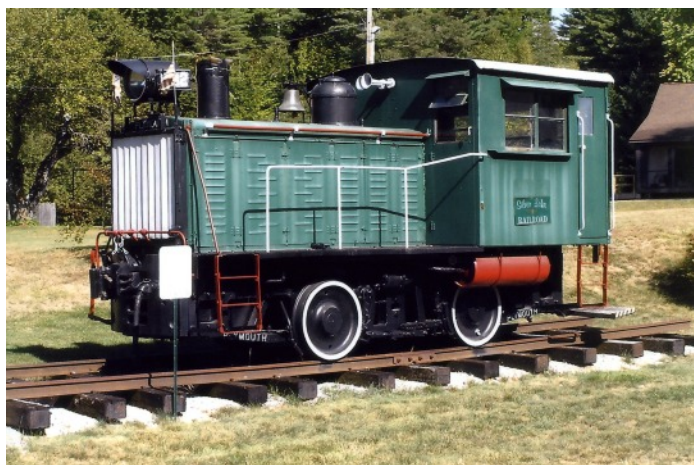
Plymouth engine used in many small industries
