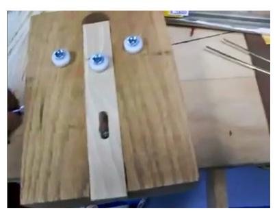
Now it looks like it has its mouth open. Well, no, that's just to show the slot in the slide to allow adjustment of the radius of curvature of the rail. Looking through the slot one can see a threaded insert to receive the thumb screw for tightening.
