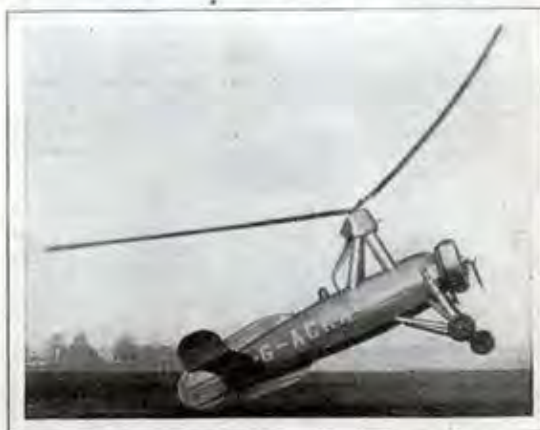
Wingless autogyro designed by Juan de la Cierva takes off for its first test at Hanworth Airport. Horizontal propellers replace wings, enabling take-off in 30 feet.
