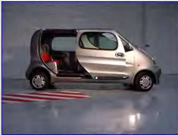
This six-seater tax, which should be available in India next year, is powered entirely by a tank filled with compressed air.
