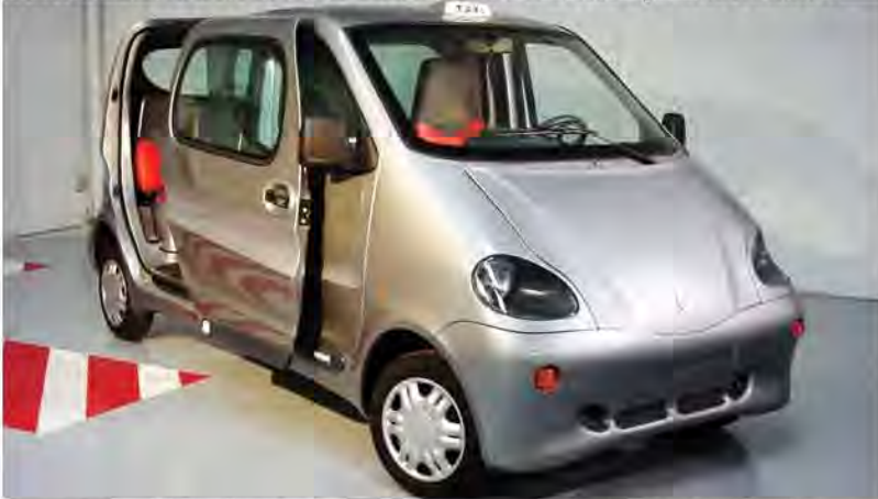
This six-seater tax, which should be available in India next year, is powered entirely by a tank filled with compressed air.
