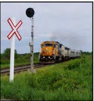
The passenger cars are re-built **GO Transit** single level cars formerly used in Toronto commuter service. The APU is a former **Milwaukee Road** "B" unit.
