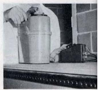
In the measurement laboratory, a technician checks the radioactivity of the radon-gas capsule with this instrument. The capsule itself is still in its lead-lined flatcar about six feet away.
