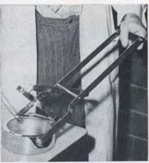
Trip to surgery is now made in hand-carried lead box, but eventually pneumatic-tube system will be used. This will still further reduce the time scientists are exposed to the deadly rays.
