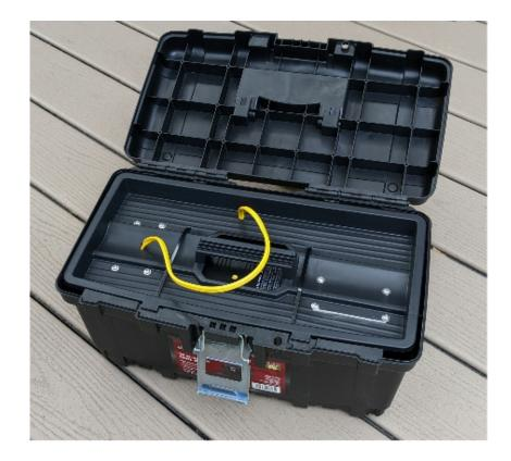
Here is the unit in "usage mode". The UP-5 is on the left, then the Zephyr, then the Powerpole jack. The power cable is visible (this was not made part of the box), and the connection from the Zephyr to the UP-5 is barely visible as well. The straps that hold the Zephyr in place are visible on either side of the unit.
