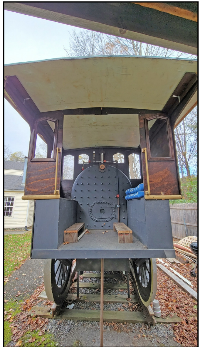
The cab details are shown in this view. The cab is constructed of wood and will support a person.
