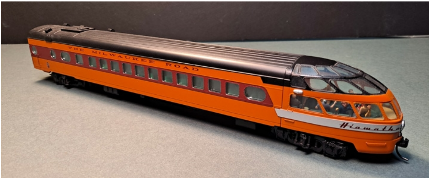
This is one of my finished models with grabs attached, tinted windows and people in the Skytop lounge. Notice the paint scheme has a black roof and only one maroon band along the windows. The lettering above the windows is also maroon in color.
